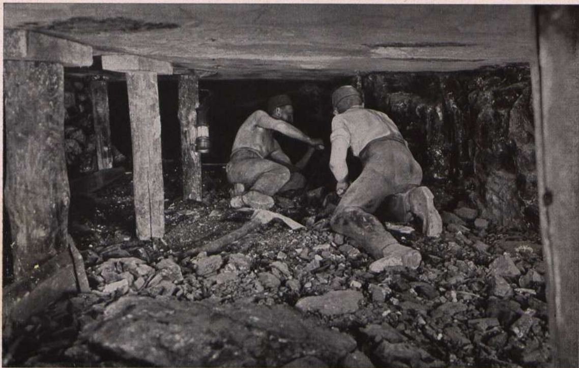
Coal mining with hand picks. Struts hold the heavy walls in place
